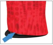
5. Feed the rubber profile in to the grove, the fabric seam make sure the fabric is even all around.
